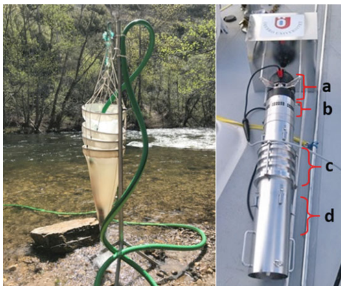
Fig. 3 Example of sampling in a river with a battery of nets with different mesh size fed by a pump with known water flow. Source: IMDEA Water (Madrid Institute for Advanced Studies on Water, Spain, left). In situ pump built by KC Denmark (Silkeborg, Denmark) and EU CleanSea project; (a) Faulhaber Swiss motor system, 3863H0224CR – 24 V, GB 150 nm with a planetary gearing 44/1–4,8:1 16 nm; (b) Water inlet with rotating blades to pull in the surrounding water; (c) stack of filters with inserted 500 \mu\text{m} , 300 \mu\text{m} , and 50 \mu\text{m} filters; (d) water outlet and flow meter (right). Source: Schönlau et al. (2020)
