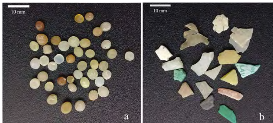
Fig. 2. Types of microplastic included in the study. (a) pre-production plastic pellets; (b) plastic fragments (mesoplastic).
